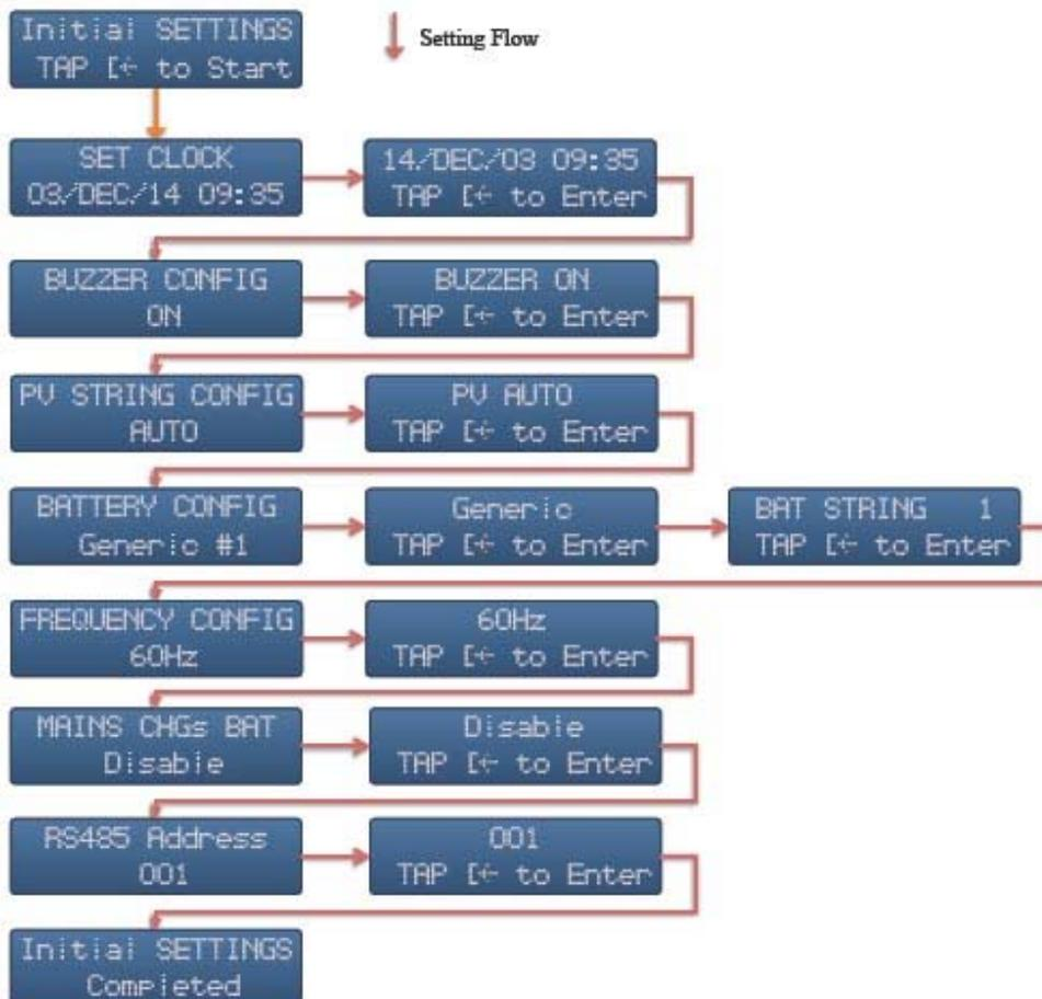
You need to set the LVS-M Series after first installation so as to have proper operation in the future. After switching on the LVS-M Series of the first installation, the initial setting frame comes out automatically. The chart is indicated.
