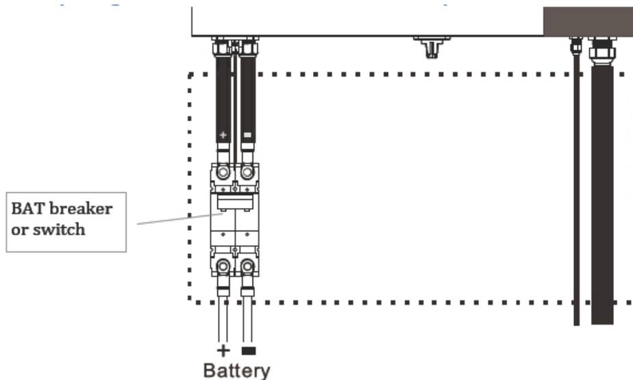
1. Select wires of cross-section >50mm. Red color is for positive (+) wire and black for negative (-).
