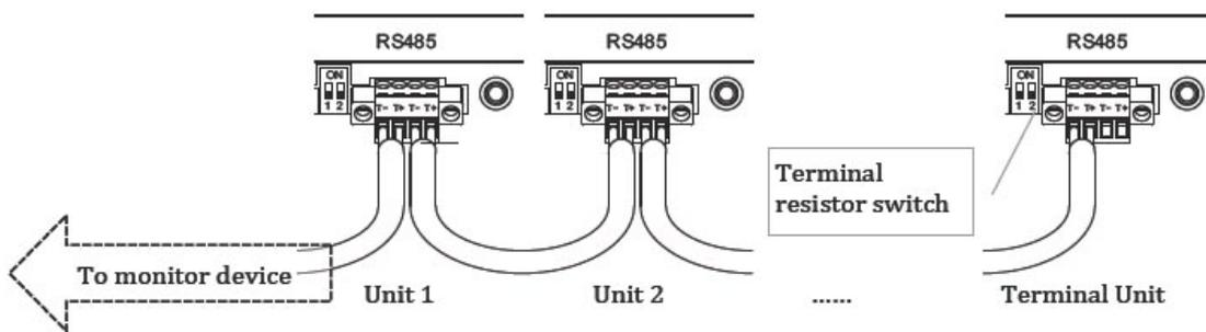
The No.2 DIP switch is the terminal resistor switch of the RS485. The default position of this switch is "off". However, if the communication does not work well, please try to switch it to "on" to improve.
