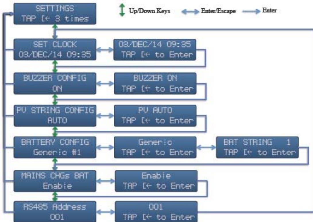
In case you would like to set the LVS-M Series, just use “Menu Up” and “Menu Down” buttons to Setting Frame and press “Confirm” button 3 times in 2 seconds to start.
