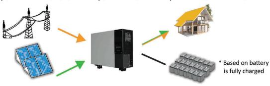
3 No PV power, no Grid power: battery supplies power for loads
