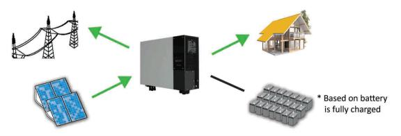
2 PV power < connected loads : PV power and Grid share power to connected loads
