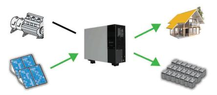
2 PV power < connected loads : PV power and battery share power to connected loads
