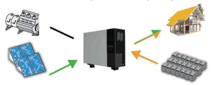
3 Battery low and PV power < connected loads : PV charges battery and generator power loads
